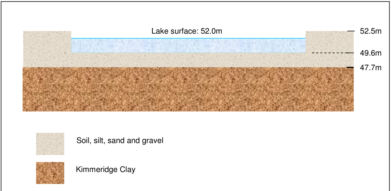
Figure 2: Schematic of vertical section of lake before filling, showing average levels (AOD) used in calculations. (Not to scale.)
